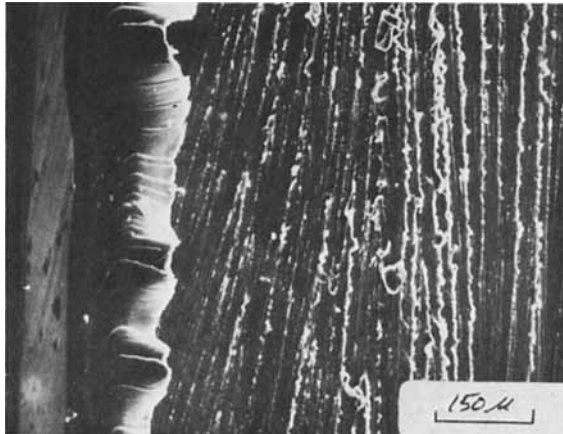
Fig. 6. Lamellar structure evident on many of the ductile fracture surfaces.
