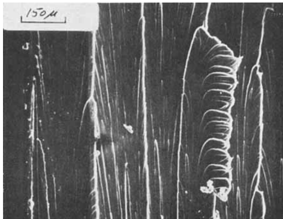
Fig. 7. Suppression of local ductility on ductile fracture surface after extended annealing.
